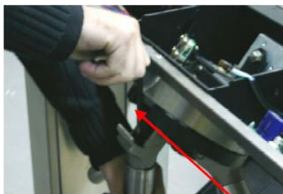
4. Fasten the screw located inside the mini-arm using a # 8 Allen wrench.
